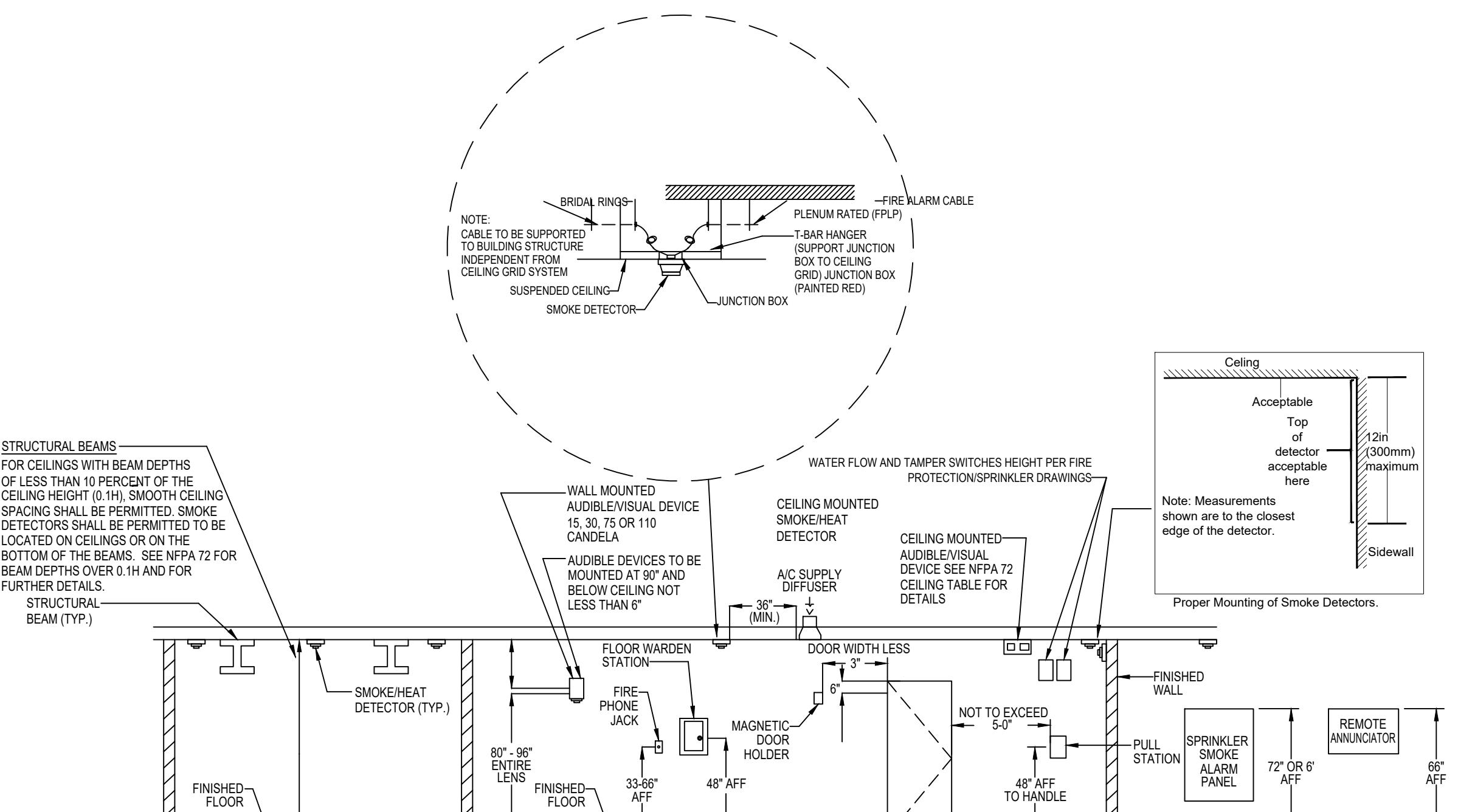
STANDARD FIRE ALARM DEVICE MOUNTING HEIGHTS
